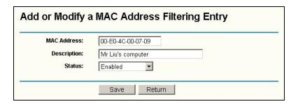
Figure 4-26 Add or Modify a MAC Address Filtering entry
