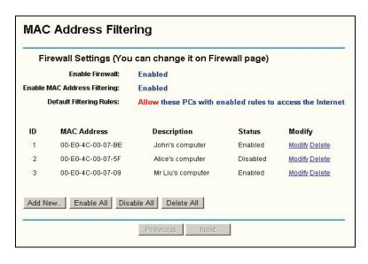
Figure 4-25 MAC Address Filtering
